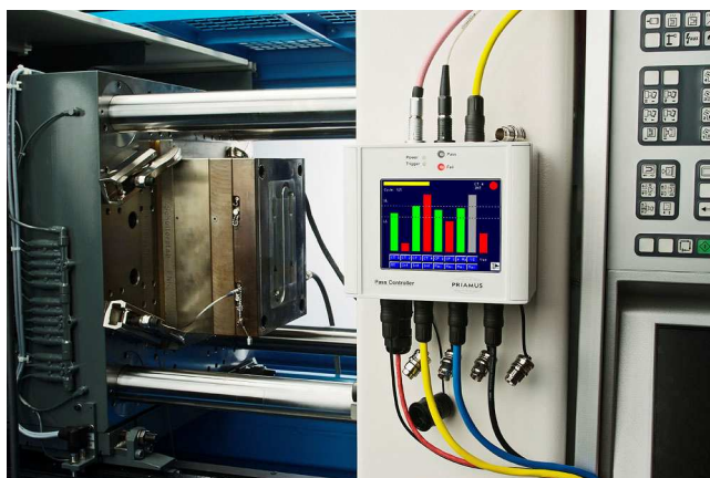
The Pass Controller with color coded connecting cables for the PDDI
