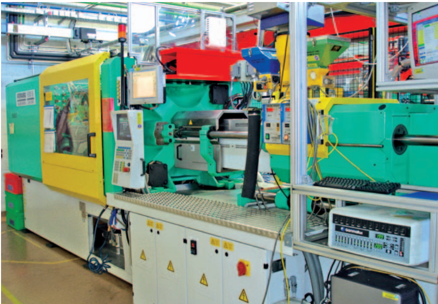
Fig. 6. The manufacturing cell for an underbody spoiler operates with the Priamus Fill hot-runner control
