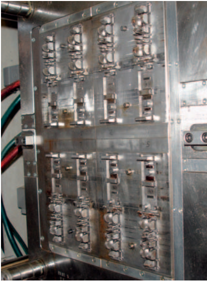
Fig. 4. The cavity temperature sensors integrated into the 8-cavity hot-runner mould automatically balance the hot runner
