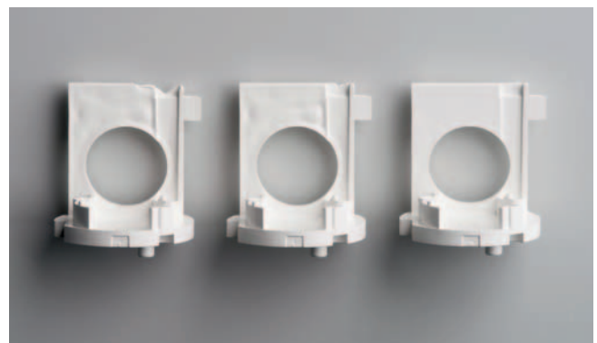
Fig. 1. When the automatic holding pressure switchover was optimized, delay times were varied between 15, 30 and 45 ms
