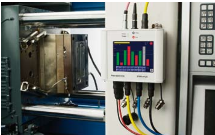
The process monitoring unit Pass Controller controls continuously the detected viscosity.
