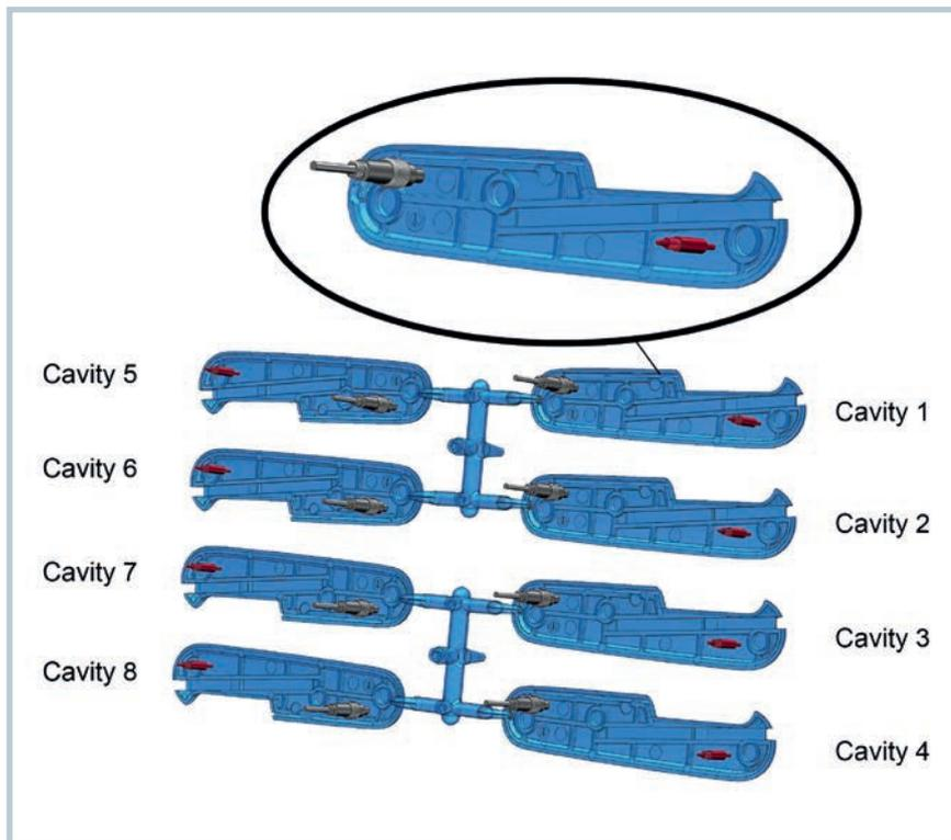
**Fig. 2.** Because the sensors in the 8-cavity mold sit in a symmetrical position, not only maximum pressures and mold temperatures can be compared directly. It is even possible to compare flow properties (viscosities) in the individual cavities
