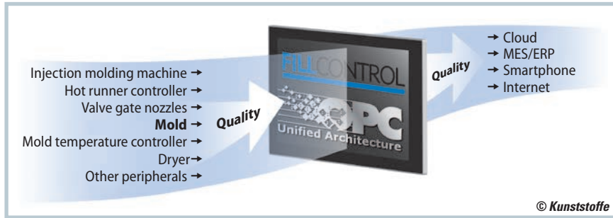
Fig. 1. The Fillcontrol process control system as a central component in the “Quality of Things”
