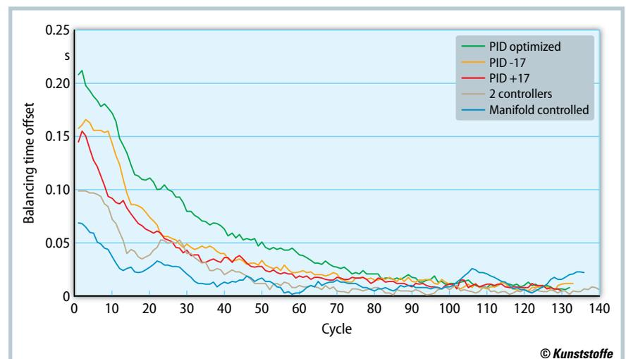
**Fig. 4.** Balancing with different PID parameter settings and control strategies. The diagram shows the temporal change in hot runner balancing based on the balancing time offset between the automatically determined temperature rises in the various cavities. The trend chart reveals the inertia of the various settings, with the smallest deviation representing the best possible balancing (source: Priamus)
