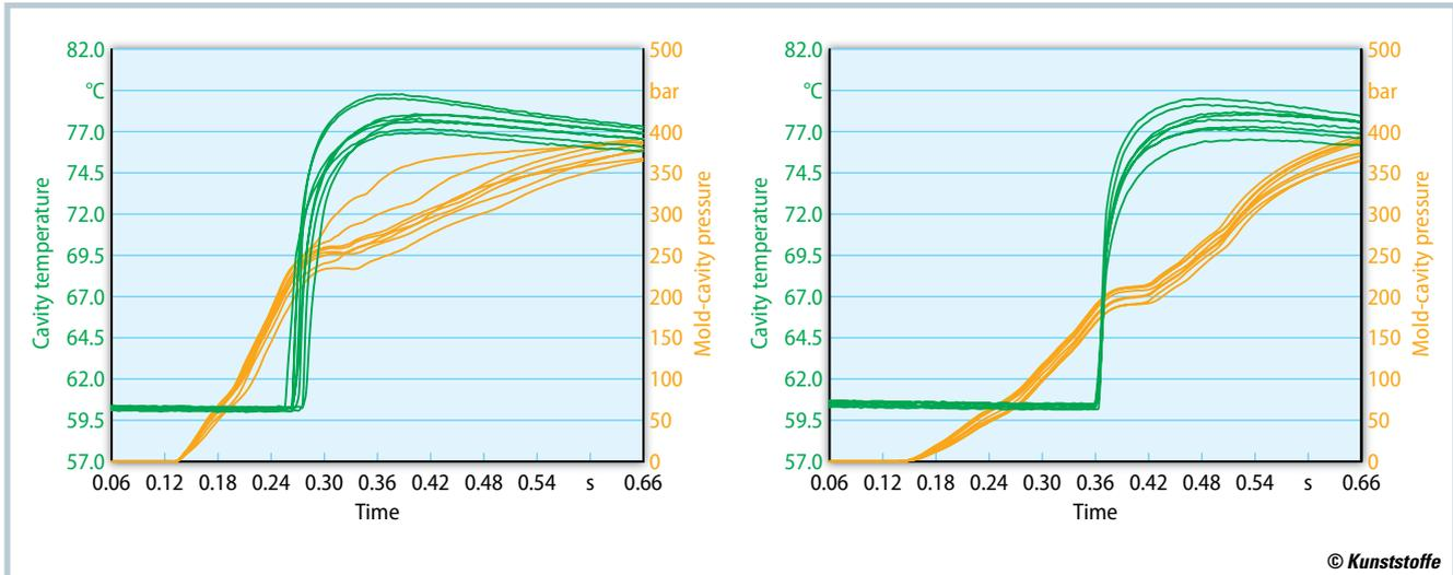
**Fig. 1.** Whereas the time offsets between the cavity pressure signals at various pressure levels differ in both the unbalanced (left) and the balanced states (right), there is virtually no time offset for the temperature rises in the balanced state (source: Priamus)
