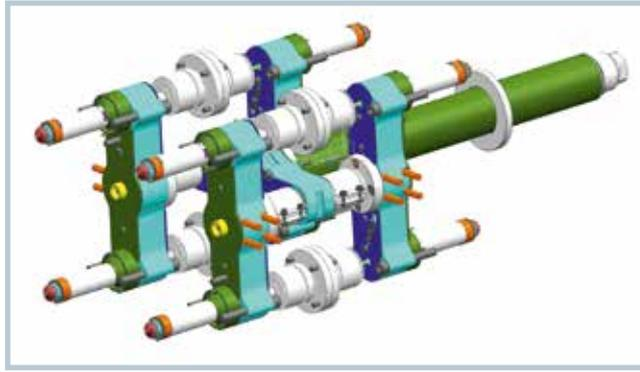
center part is a potential weak point that can lead both to variations in part quality within a single shot and to increased wear. As the center part is usually not very rigid and is not supported by the clamping platens, it can deform under the influence of the clamping force and the injection pressure. This, along with process influences, can contribute to uneven mold filling.
