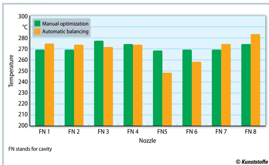
**Fig. 5.** While a balancing time offset of 0.1 s was recorded for manual optimization, a time offset of just 0.01 s was achieved with automatic balancing. For optimal balancing, the nozzle temperatures had to be adjusted accordingly (source: Priamus)
