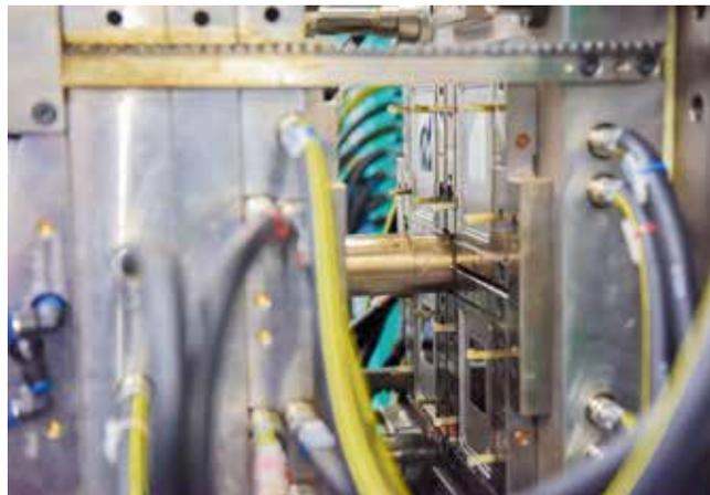
**Fig. 2.** View inside the stack mold. The rack and the melt guide tube are clearly visible (© Priamus)
